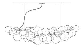
Configuration 02 ADJUSTABLE STEEL CABLE SUSPENSION / CENTER JUCTION BOX
